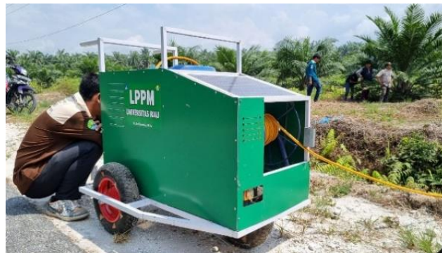
Gambar 2 : Alat Smart Gun Sprayer Pengendalian Gulma Berbasis Ergonomi
