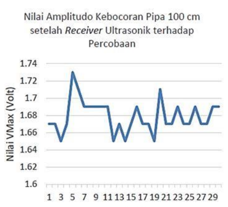
Figure 6: data for the amplitude value of the leaking pipe condition 100 cm after the ultrasonic receiver.
