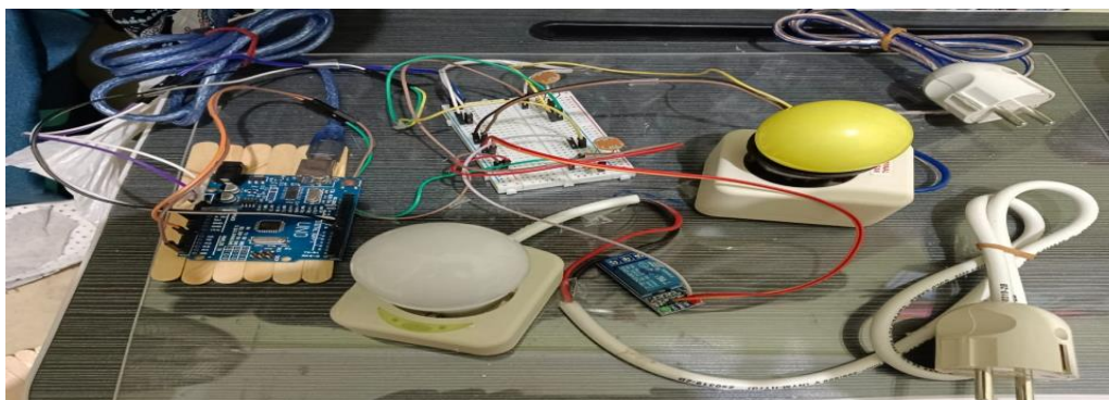
Figure 3 : A Simple On / Off controller circuit using a relay based on LDR sensor and Arduino Uno
