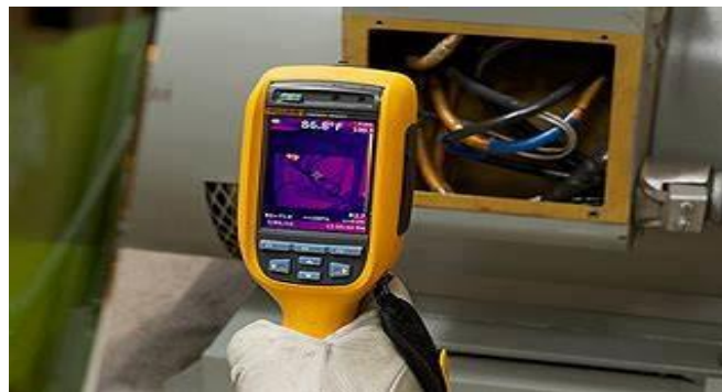
Figure 5. Thermal Infrared (IRT) Testing
