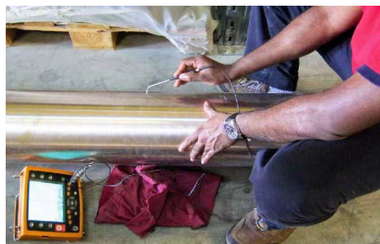
Figure 3. Eddy Current Testing (ECT)
