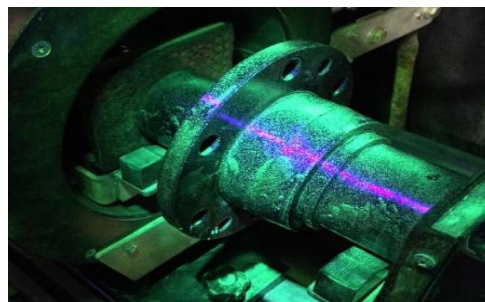
Figure 2. Magnetic Particle Inspection (MPI)
