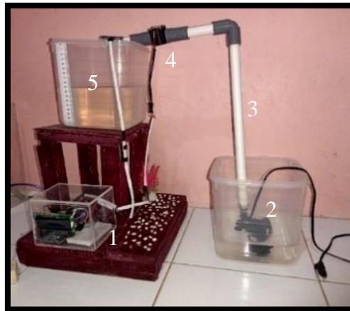
1. Tool box (Lcd , Buzzer, Beardboard, Arduino Uno), 2. Aquarium water pump and water reservoir, 3. Pipe 3,2 cm 2 and 1.6 cm 2 , 4. Water Flow Sensor, 5. Water reservoir and Ultrasonic sensor
