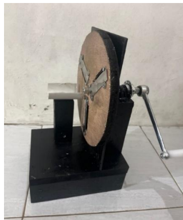
Figure 2. Design of the manual potato slicer prototype.
